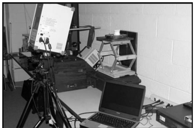
FIG. 1—The 3D digitization setup with the Minolta VIVID 910 non-contact 3-D digitizer (the white rectangular box on the left) and the rotating platform with the dental cast on it.
